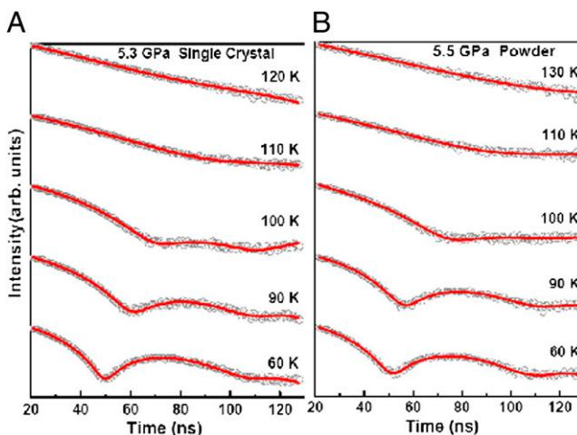
**Fig. 1.** Representative temperature-dependent SMS spectra of  $\text{BaFe}_2\text{As}_2$  in Ne pressure medium. (A) Single crystal at 5.3 GPa. (B) Powder sample at 5.5 GPa.  $\circ$ , experimental data; red solid lines, modeled spectra using the CONUSS program. Quantum beats in the spectra represent the occurrence of the magnetic fields and hence the AFM state, whereas the absence of beats (flat spectral feature) indicates the PM state.
