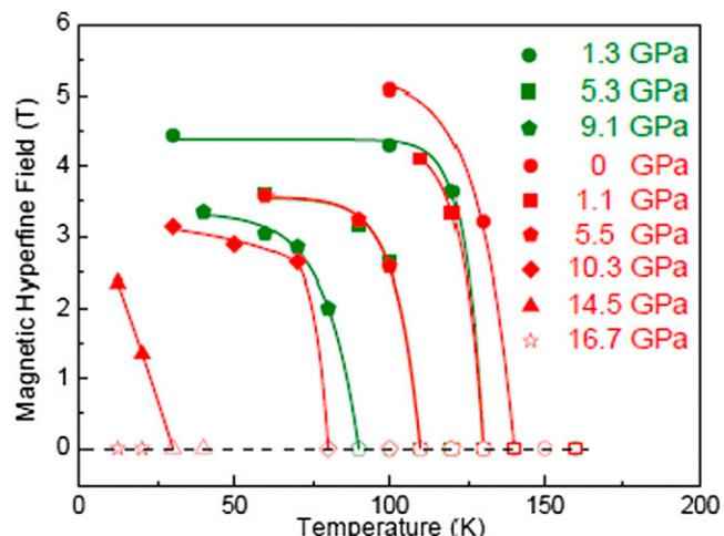
**Fig. 2.** Derived hyperfine magnetic fields of  $\text{BaFe}_2\text{As}_2$  as a function of temperature at high pressures. Red symbols, powder in Ne medium; olive symbols, single crystal in Ne medium; solid symbols, AFM state; open symbols, PM state; solid lines, simple fitting to the data.
