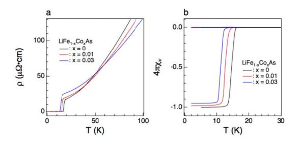
Supplementary Figure 1: Resistivity and magnetic susceptibility of  $LiFe_{1-x}Co_xAs$ . Supplementary Figures 1a and 1b show the resistivity and the magnetic susceptibility of  $LiFe_{1-x}Co_xAs$ . The low residual resistivity and high superconducting (SC) volume prove the high quality of our samples.
