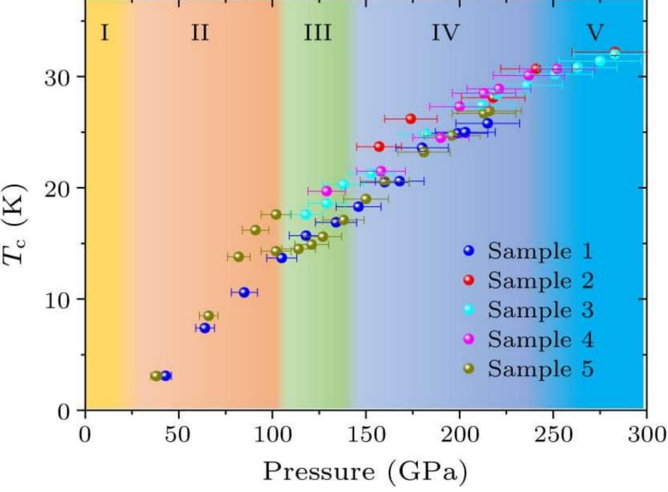
Scandium is the only known elemental superconductor to have a critical temperature in the 30 K range. This phase diagram shows the superconducting transition temperature ( $T_c$ ) and crystal structure versus pressure for scandium. The measured results on all the five samples studied show consistent trends. (Courtesy: <u>Chinese Phys. Lett. **40**</u> 107403)
