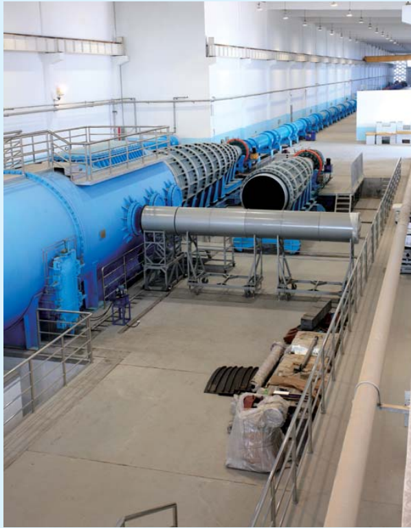
Hypersonic Flight Conditions Duplicating Shock Tunnel
