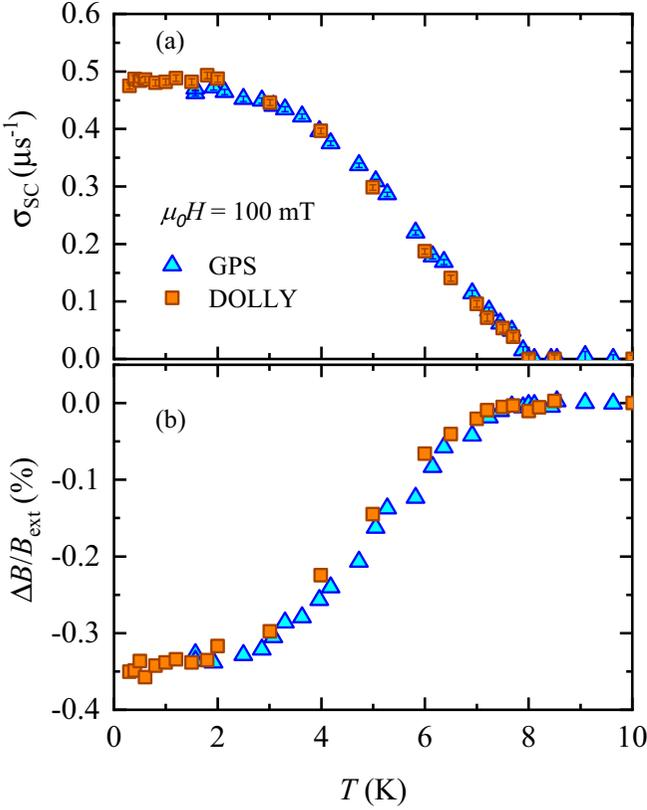
FIG. 4. (a) Temperature dependence of the superconducting muon-spin depolarization rate  $\sigma_{\text{SC}}$  of ZrRuAs measured in an applied magnetic field of  $\mu_0 H = 100$  mT. (b) Temperature dependence of the relative change of the internal field normalized to the external applied field,  $\Delta B/B_{\text{ext}}$  ( $= \frac{B_{\text{int}} - B_{\text{ext}}}{B_{\text{ext}}}$ ).
