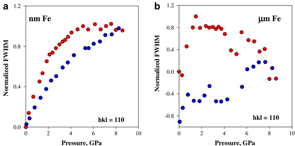
Fig. 2. Peak width vs. pressure for nano-Fe (a) and micro-Fe (b). The red circles are for the pressure loading process and the blue circles indicate the unloading process. (For interpretation of the references to color in this figure legend, the reader is referred to the web version of this article.)
