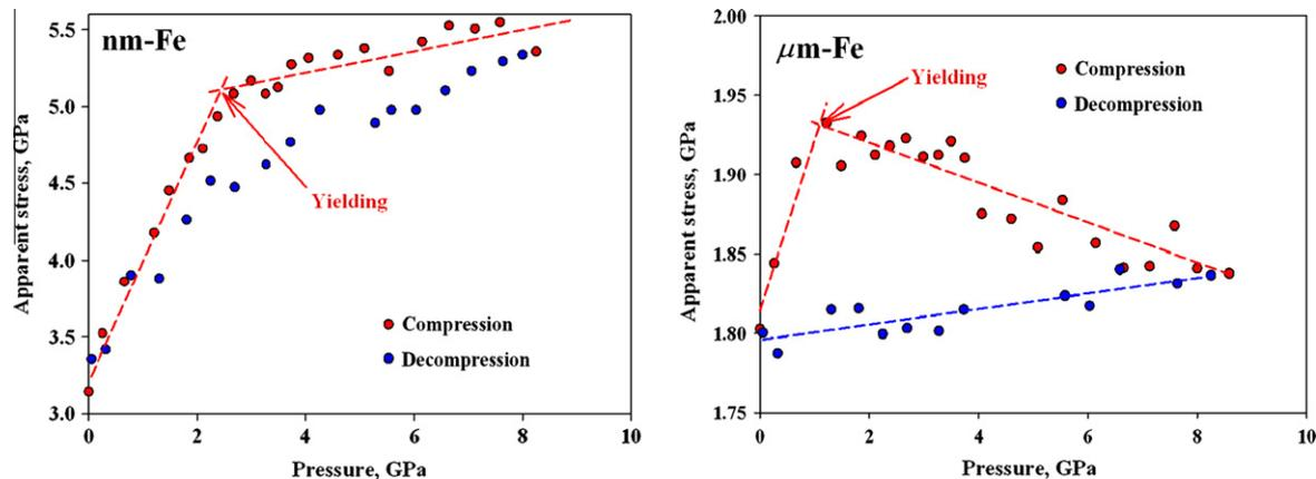
Fig. 4. Apparent stresses of nano-Fe and micro-Fe plotted as a function of pressure, which includes both microstrain and instrument-zero effects. The “yielding” points are derived from the intersections of elastic loading and plastic work-hardening/softening stages.
