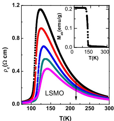
FIG. 1. (Color online) Temperature dependence of  $c$ -axis resistivity ( $\rho_c$ ) for LSMO single crystal for different pressures ( $P$ ). Inset: Temperature dependence of in-plane magnetization at  $H=0.01$  T. The arrow indicates the direction of increase in  $P$ .
