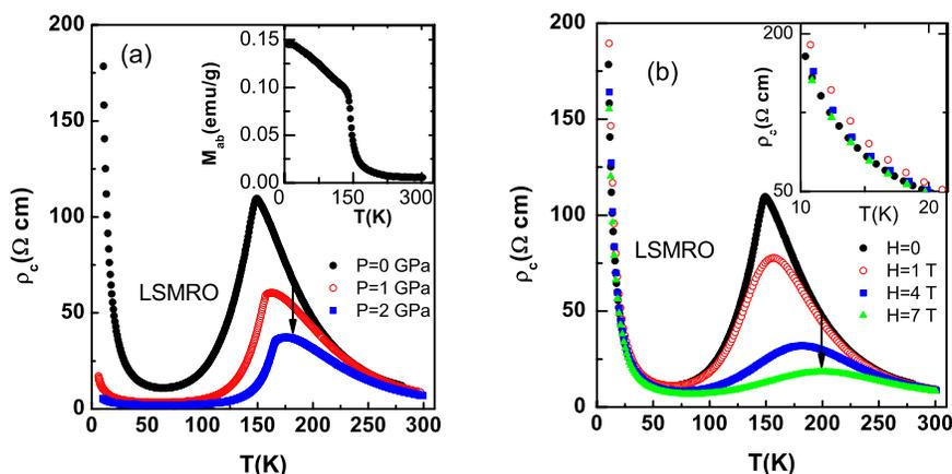
FIG. 2. (Color online) (a) Temperature dependence of  $c$ -axis resistivity ( $\rho_c$ ) for LSMRO single crystal for different pressures ( $P$ ). The inset shows the temperature dependence of in-plane magnetization at  $H=0.01$  T. (b) Temperature dependence of  $\rho_c$  for LSMRO single crystal for different magnetic fields at ambient pressure. The inset shows  $T$  dependence of  $\rho_c$  below 20 K for different  $H$ . The arrows indicate the direction of increase in  $P$  and  $H$ .
