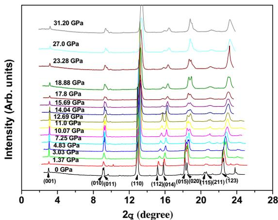
Fig. 2. Angle-dispersive X-ray diffraction spectra for NdBa<sub>2</sub>Cu<sub>3</sub>O<sub>6+δ</sub> sample at room temperature.
