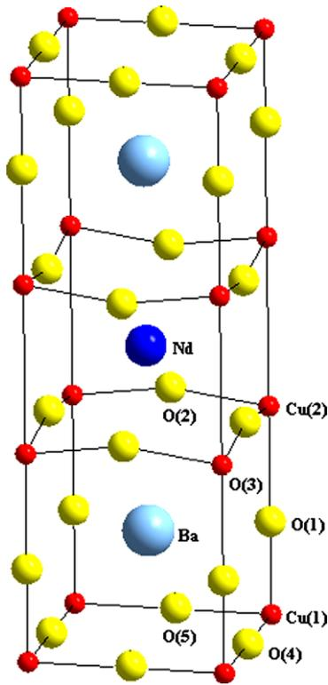
Fig. 1. Schematic view of the crystal structure of NdBa<sub>2</sub>Cu<sub>3</sub>O<sub>6+δ</sub>.
