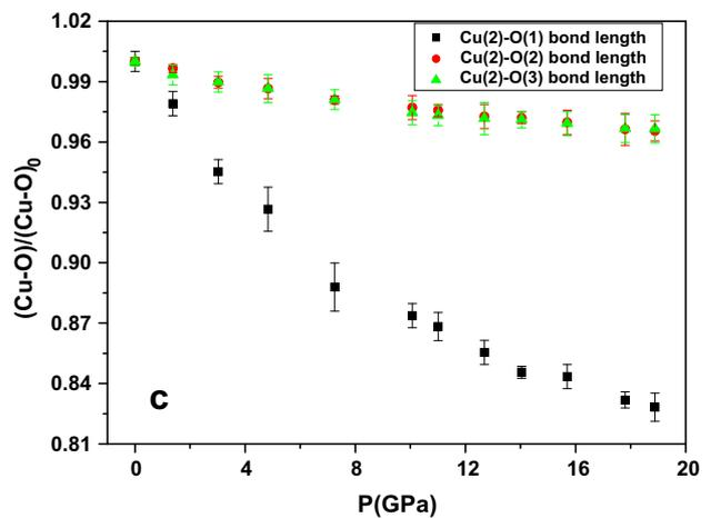
Fig. 3. The relationship of lattice parameters (a), volume compressibility (b) and Cu(2)–O(1), Cu(2)–O(2) and Cu(2)–O(3) bond length compressibility (c) versus pressure for NdBa<sub>2</sub>Cu<sub>3</sub>O<sub>6+δ</sub> sample.
