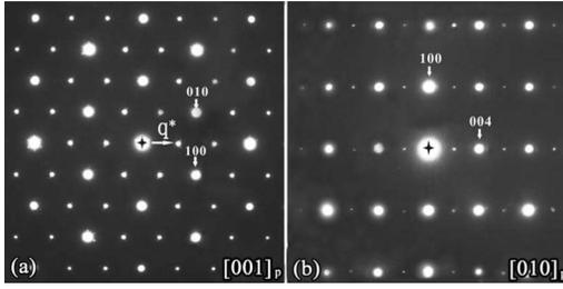
FIG. 1. Selected area ED patterns of  $\text{Sr}_{0.39}\text{CoO}_2$  along the (a)  $[001]_p$  and (b)  $[010]_p$  zone-axes.
