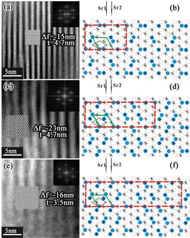
FIG. 3. (Color online) (a), (c), and (e) are the HRTEM images of  $3\sqrt{3}a_p \times 3a_p$ ,  $5\sqrt{3}a_p \times 3a_p$ , and  $7\sqrt{3}a_p \times 3a_p$  modulated phases along the  $[001]_p$  zone axis, respectively. (b), (d), and (f) are the corresponding structure models in  $\mathbf{a}_p$ - $\mathbf{b}_p$  plane, where the supercell is marked by dashed lines (red ones in color figure).
