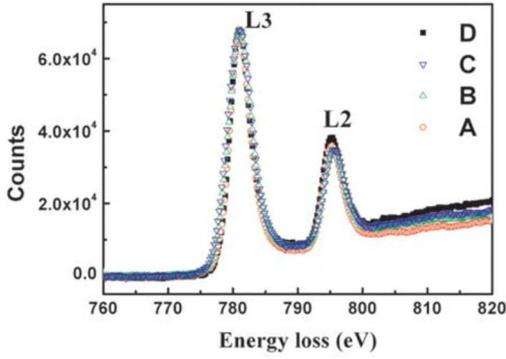
FIG. 4. (Color online) Normalized EELS spectra including Co- $L_{2,3}$  edges obtained from different modulated phases along the  $[001]_p$  zone-axis direction, where A, B, C, and D denote  $\sqrt{3}a_p \times \sqrt{3}a_p$ ,  $7\sqrt{3}a_p \times 3a_p$ ,  $5\sqrt{3}a_p \times 3a_p$ , and  $3\sqrt{3}a_p \times 3a_p$ , respectively.
