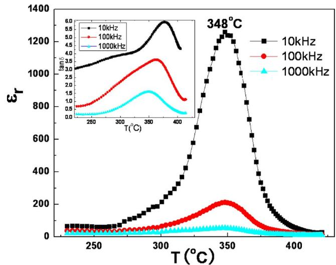
FIG. 2. (Color online) The temperature dependence of dielectric constant and loss of  $\text{TmMnO}_3$  measured at different frequencies of 10, 100, and 1000 kHz. Inset: the inverse dielectric constant and high- $T$  Curie-Weiss fit (red solid line).
