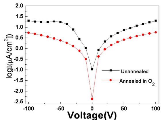
FIG. 3. (Color online) Logarithm of leakage current  $I$  vs applied voltage  $V$  for thin plate  $\text{TmMnO}_3$  ceramics (solid square: unannealed, solid circle: annealed in  $\text{O}_2$  at 500 °C for 8 h).
