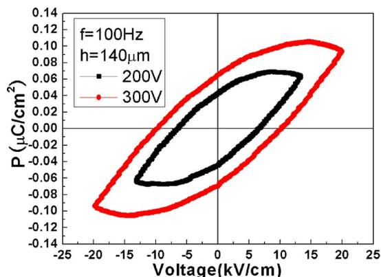
FIG. 4. (Color online) Polarization-electric field hysteresis loop collected at different applied fields and at a frequency of 100 Hz.
