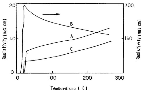
FIG. 1. Resistance dependence on temperature: (a) high-pressure sintered bulk, (b) conventional bulk, (c) the single crystal.
