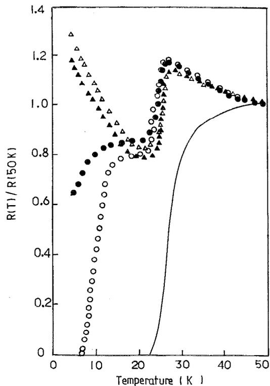
FIG. 3. Resistance dependence on temperature for a typical conventional bulk at different measuring currents: 10  $\mu\text{A}$  ( $\circ$ ), 100  $\mu\text{A}$  ( $\bullet$ ), 1 mA ( $\blacktriangle$ ), 10 mA ( $\triangle$ ), and the high-pressure sintered sample (solid line).
